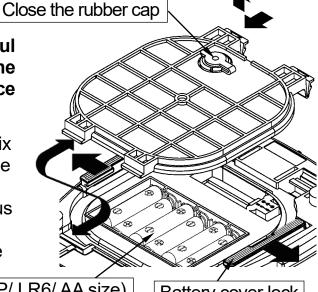
New six batteries (R6P/ LR6/ AA size)
